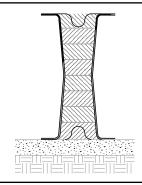
Fill Cones in 6" layers from the bottom up, compact each layer. Use recommended backfill material.
